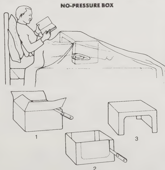
No-pressure box: this device lifts blankets and sheets off the patient. Get a medium-size cardboard box and cut in the shape of a table.
